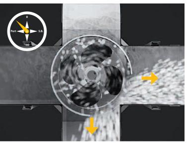
For our 2-channel version we have developed a system in which the steering angle of the drum and the speed of the diesel engine is continuously variable in a setup using one infinitely adjustable handle (which moves from side to side, like a tunnel). The operation is thus highly effective and very responsive!
