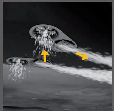
With the aid of a horizontal propeller, the water is drawn in from under the vessel. Then the water is guided via a hydro-dynamically streamlined house to the outside through a grid. This grid is steerable through 360°.
